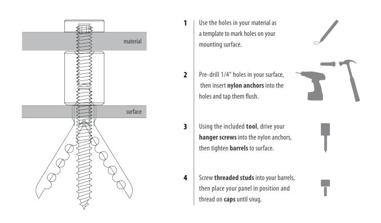
TIP 1: A wood hanger screw driver tool is included to drive the screw into the nylon anchor or wood. TIP 2: We recommend 7/32" holes in your material to give you more freedom for aligning your panels. MADE IN USA
