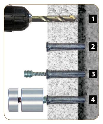
(1) With a masonry bit, pre-drill a 1/4" diameter hole x 1-1/2" deep in concrete, cinder block or other masonry surface.
