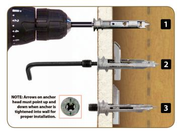
(1) With a Phillips Bit, self-drill the anchors into position (please see notation on diagram). NOTE: *These anchors are intended for hollow walls* 1/2" - 3/4" thick.
