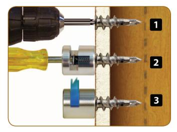
(1) With a Phillips Bit, self-drill the anchors into position. NOTE: *These* anchors are not intended for wood or other dense materials. Intented for 1/2" or thicker drywall.
