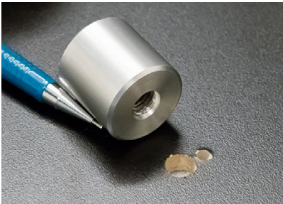
Place the barrel to mark holes for mounting hardware and wiring. Drill 11/32" for anchoring center and 5/32" for wiring hole.
